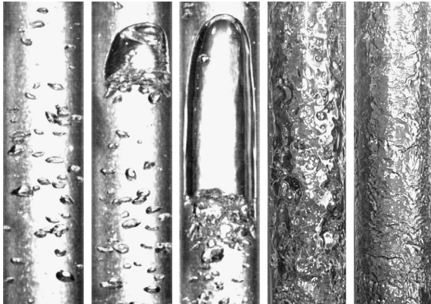
Fig. 1. Typical air–water flow images observed in a vertical upward two-phase flow in a pipe of 25.4 mm diameter.
